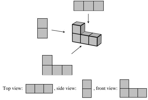
An object has the following top view and front view:
