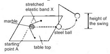
She stretched an elastic band X and placed a marble against it. She released the marble to hit the steel ball, causing the steel ball to swing upwards.
