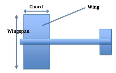
1. The diagram shows a view of a model glider from above.
