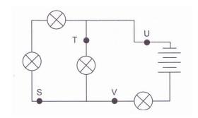
Darcy wants to install a switch so that he is able to switch off TWO bulbs while leaving the rest of the bulbs lighted. Which part of the circuit S, T, U or V should Darcy install the switch? (1 point)
